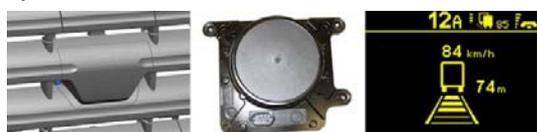
The driver sets a desired cruise speed and following distance mode to a vehicle ahead. ACC adapts the vehicle's speed to maintain the preset following distance.
